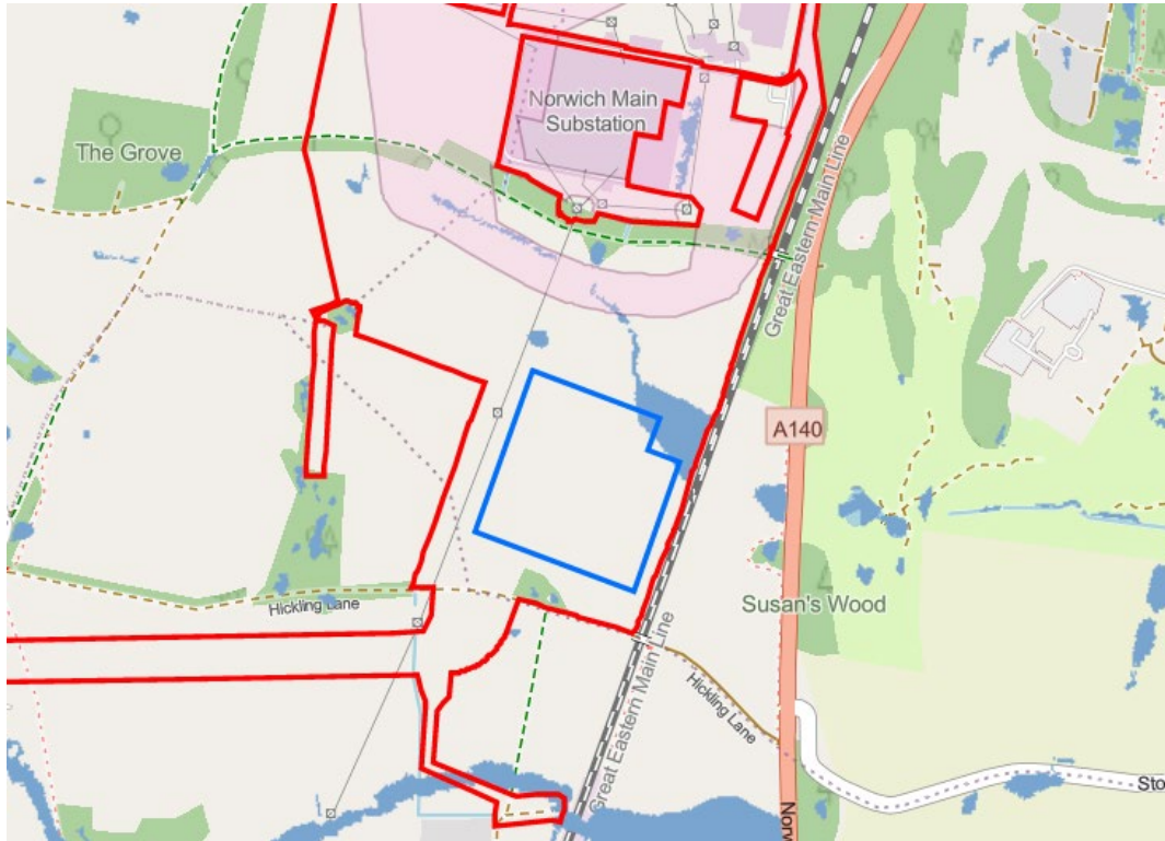
Plate 3-3: Preferred substation footprint (Royal blue boundary) taken forward for the DCO application. Areas of potential surface water flood risk (identified within the Environment Agency held dataset) associated with naturally low lying areas shown as lighter blue areas.
